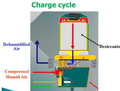
Figure 8 Schematic of Generation Cycle [4]
