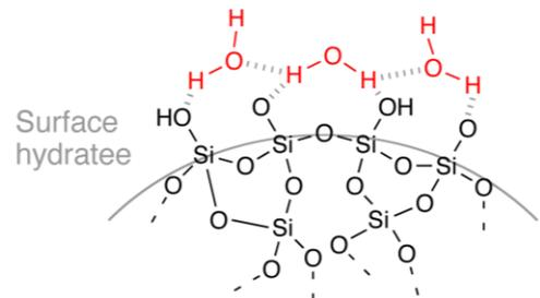
Figure 7 Surface Hydrate of Silica Gel
