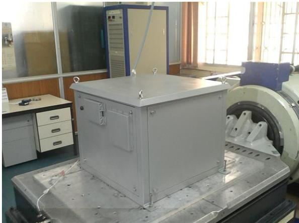
Figure 12 APS under testing (Vibration test)
