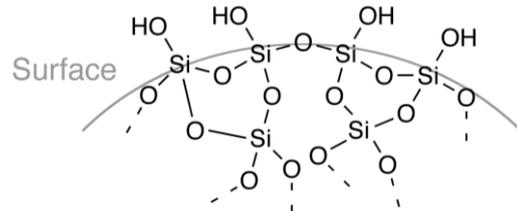
Figure 6 Surface of Silica Gel
