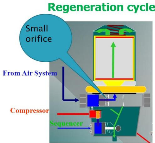
Figure 9 Schematic of Regeneration cycle [4]
