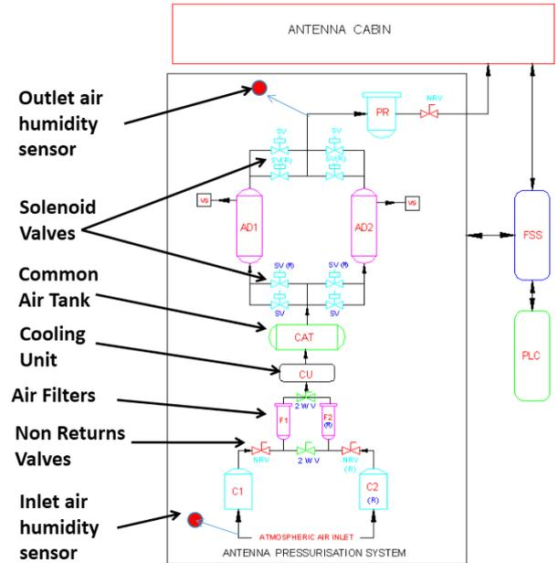
Figure 10 Schematic diagram of Antenna Pressurisation System
