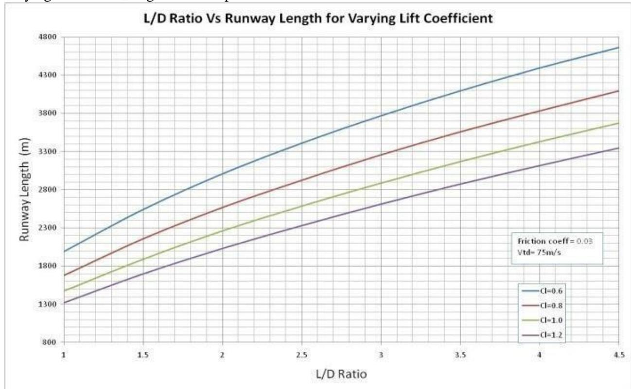
**Graph 1: Variation of L/D ratio vs Runway length for varying Lift coefficient ( $C_L$ ).**
