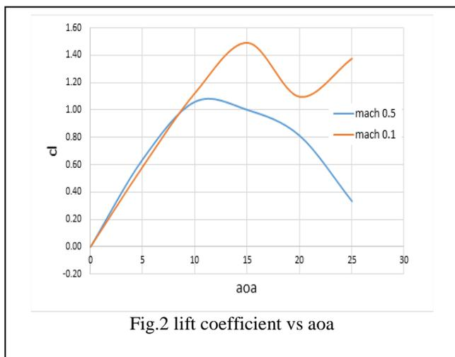
Fig.2 lift coefficient vs aoa
