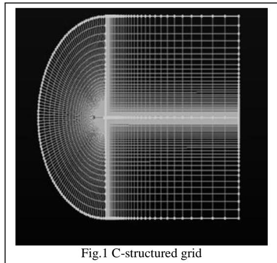
Fig.1 C-structured grid
