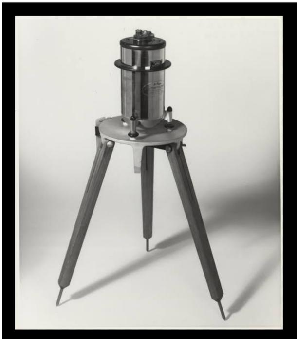
The gravity M is a sensitive instrument which can measure the difference in  $g$  values at different places. Various principles have been used in their construction and instruments of various ranges from 5000 mgal to 30 mgal, developed.
